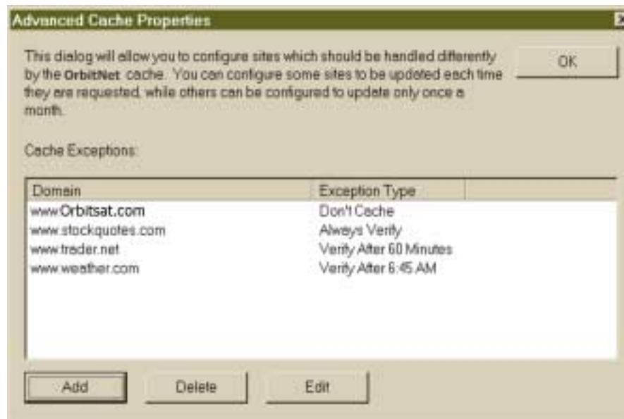
Figure 9-22: With advanced cache, you can configure the way in which specific sites are handled by OrbitNet's Web cache.
