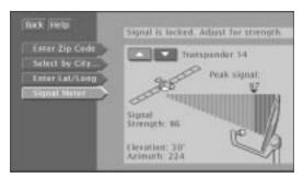
If the satellite dish antenna is pointed to the correct azimuth and elevation, the signal meter will show you the current signal strength (and you should hear a continuous tone).
